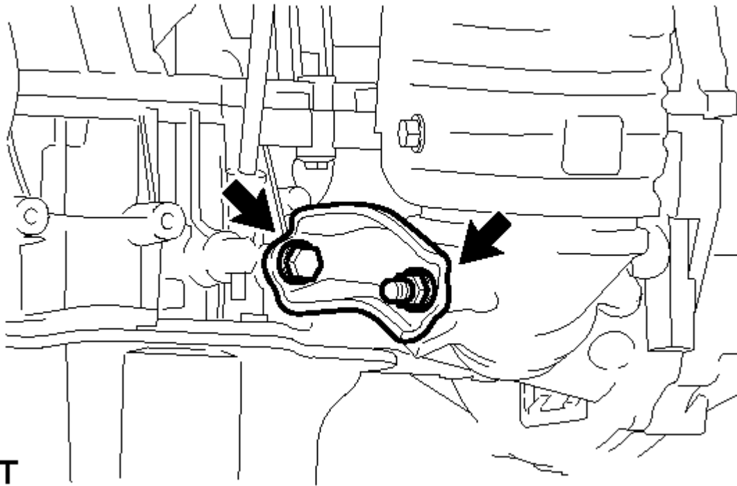
Fig. 143: Locating Manifold Stay Bolt And Nut Courtesy of TOYOTA MOTOR SALES, U.S.A., INC.
