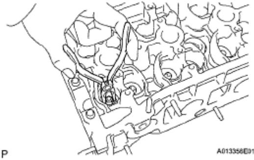
Fig. 151: Identifying Oil Seals Using Needle Nose Pliers Courtesy of TOYOTA MOTOR SALES, U.S.A., INC.
