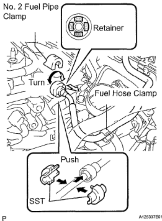
Fig. 293: Turning SST To Align Retainer Inside Fuel Tube Connector Courtesy of TOYOTA MOTOR SALES, U.S.A., INC.
