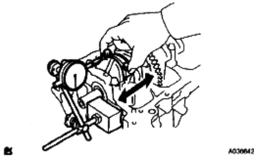
Fig. 212: Measuring Thrust Clearance While Moving Connecting Rod Back And Forth Courtesy of TOYOTA MOTOR SALES, U.S.A., INC.
