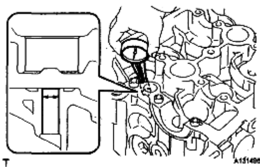
Fig. 177: Measuring Bush Bore Diameter Of Cylinder Head Courtesy of TOYOTA MOTOR SALES, U.S.A., INC.
