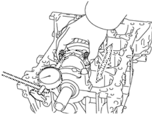
Fig. 302: Measuring Connecting Rod Thrust Clearance Courtesy of TOYOTA MOTOR SALES, U.S.A., INC.
