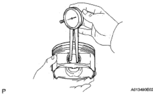
Fig. 305: Identifying Piston Pin Bore Diameter
