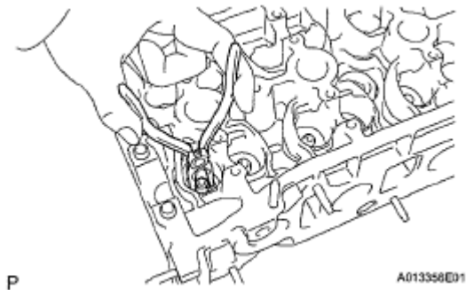
Fig. 145: Identifying Oil Seals Using Needle-Nose Pliers Courtesy of TOYOTA MOTOR SALES, U.S.A., INC.
