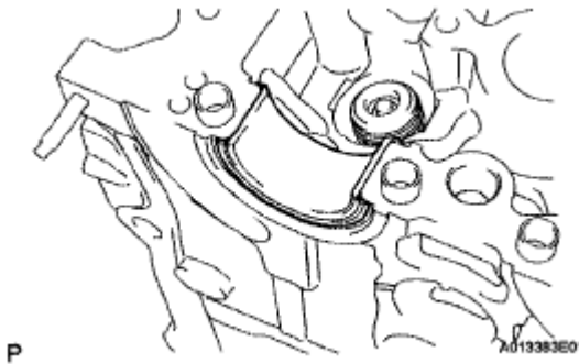
Fig. 192: Identifying Camshaft Bearing Onto Cylinder Head
