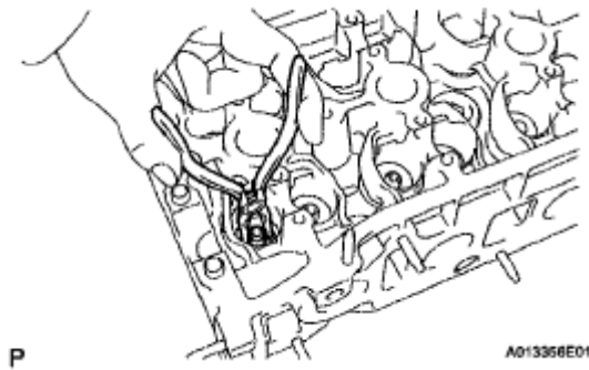
Fig. 145: Removing 16 Oil Seals Using Needle-Nose Pliers
