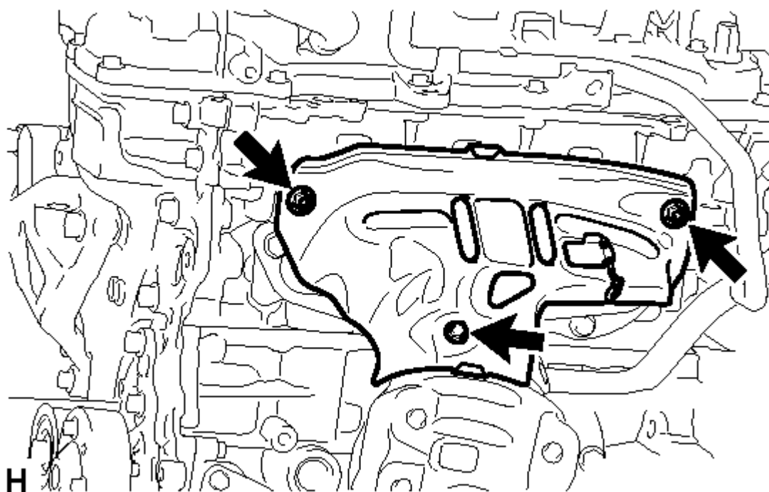
Fig. 134: Identifying Exhaust Manifold Heat Insulator Nuts & Bolt
