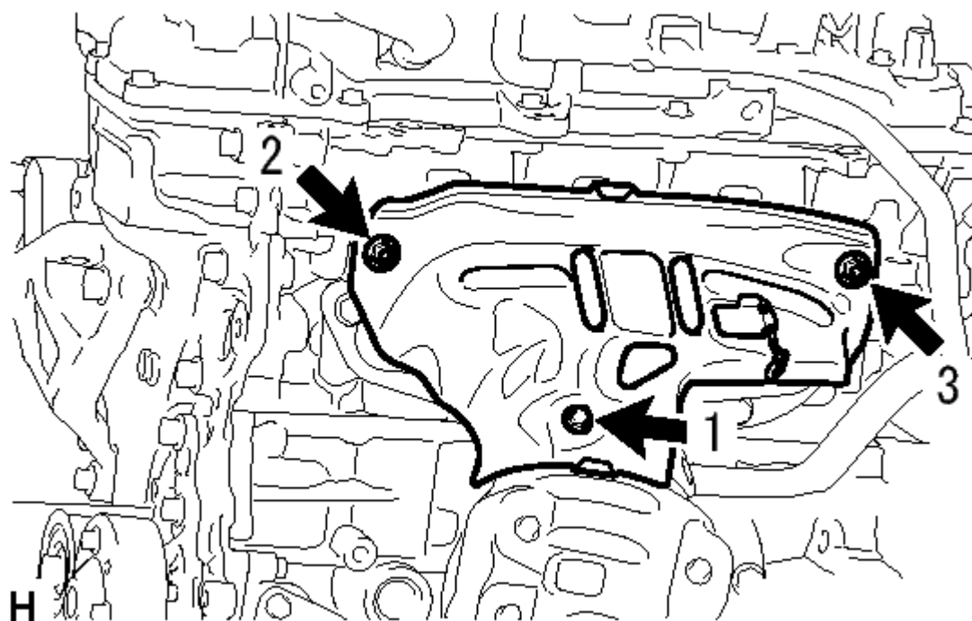
Fig. 314: Identifying Exhaust Manifold Heat Insulator Nuts And Bolt Courtesy of TOYOTA MOTOR SALES, U.S.A., INC.
