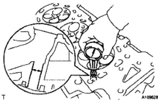
Fig. 146: Checking Bush Bore Diameter Of Cylinder Head
