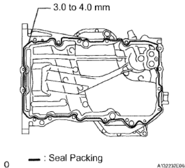
Fig. 599: Identifying Oil Pan Seal Packing Area
