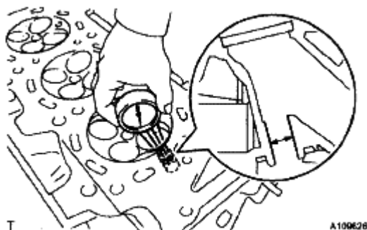
Fig. 143: Checking Bush Bore Diameter Of Cylinder Head Courtesy of TOYOTA MOTOR SALES, U.S.A., INC.
