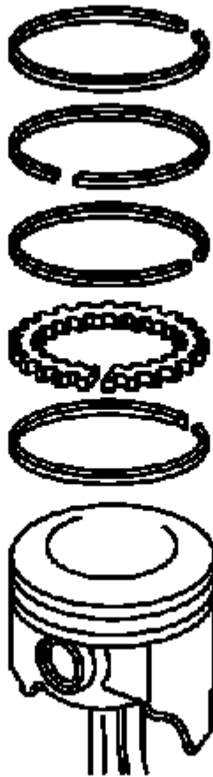
Fig. 353: Exploded View Of Piston Rings Courtesy of GENERAL MOTORS CORP.
