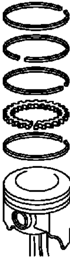
Fig. 340: Exploded View Of Piston Rings Courtesy of GENERAL MOTORS CORP.
