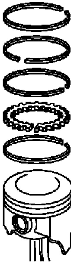
Fig. 355: Exploded View Of Piston Rings Courtesy of GENERAL MOTORS CORP.
