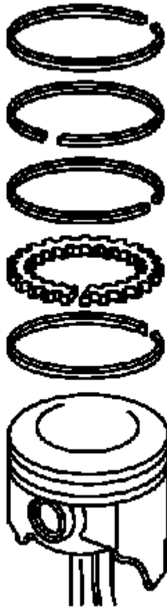
Fig. 428: Exploded View Of Piston Rings Courtesy of GENERAL MOTORS CORP.
