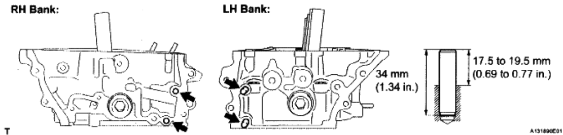
Fig. 359: Identifying Straight Pin Position Courtesy of TOYOTA MOTOR SALES, U.S.A., INC.
