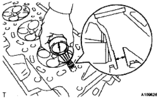
Fig. 349: Checking Bush Bore Diameter Of Cylinder Head Courtesy of TOYOTA MOTOR SALES, U.S.A., INC.
