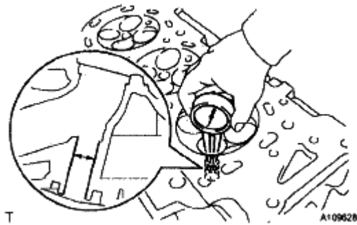
Fig. 352: Checking Bush Bore Diameter Of Cylinder Head
