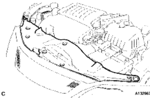
Fig. 34: Identifying Clips And Intake Duct Seal Courtesy of TOYOTA MOTOR SALES, U.S.A., INC.
