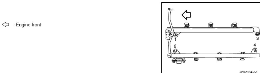
Fig. 62: Identifying Tightening Sequence Of Fuel Tube And Fuel Injector Assembly Courtesy of NISSAN NORTH AMERICA, INC.
