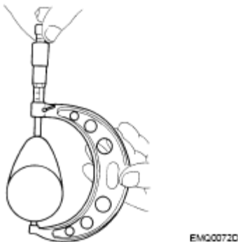
Fig. 137: Checking Camshaft Cam Height Courtesy of NISSAN MOTOR CO., U.S.A.
