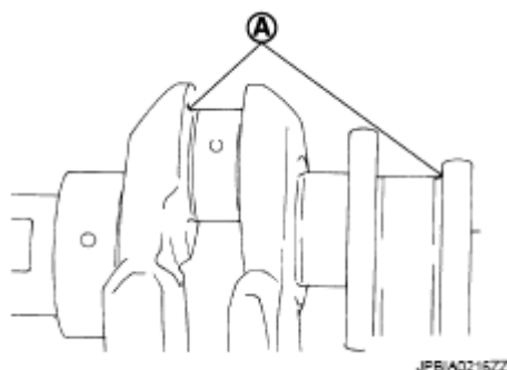
Fig. 255: Identifying Crankshaft Pin Courtesy of NISSAN MOTOR CO., U.S.A.
