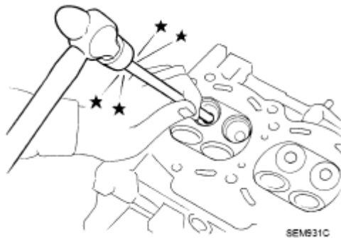
Fig. 150: Driving Out Valve Guide Courtesy of NISSAN MOTOR CO., U.S.A.
