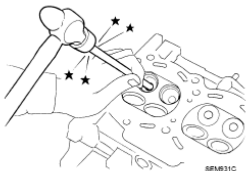
Fig. 204: Driving Out Valve Guide Courtesy of NISSAN NORTH AMERICA, INC.
