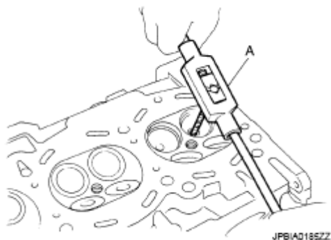
Fig. 205: Reaming Cylinder Head Valve Guide (EXH) Hole Using Valve Guide Reamer Courtesy of NISSAN NORTH AMERICA, INC.
