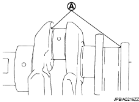
Fig. 285: Identifying Fillet Area Crankshaft Courtesy of NISSAN NORTH AMERICA, INC.
