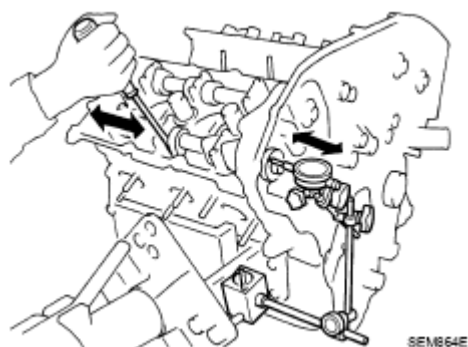
Fig. 184: Measuring Camshaft End Play Using Dial Indicator Courtesy of NISSAN NORTH AMERICA, INC.
