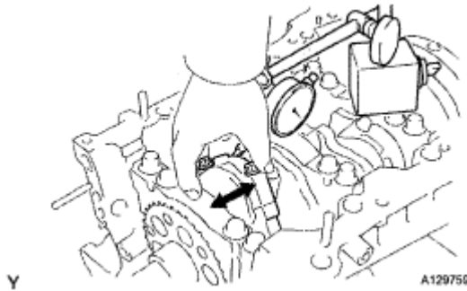
Fig. 266: Measuring Thrust Clearance While Moving Connecting Rod Back And Forth Courtesy of TOYOTA MOTOR SALES, U.S.A., INC.
