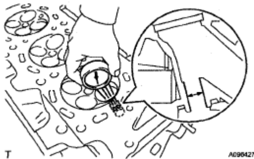
Fig. 314: Measuring Bush Bore Diameter Of Cylinder Head
