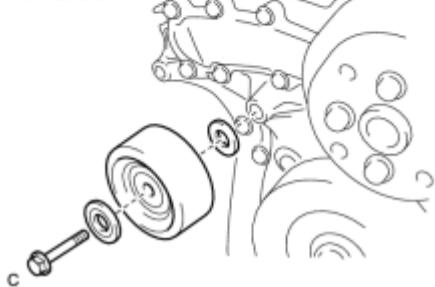
Fig. 72: Locating No. 2 Idler Pulley Sub-Assembly Bolts Courtesy of TOYOTA MOTOR SALES, U.S.A., INC.
