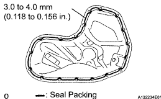
Fig. 430: Applying Seal Packing In Continuous Bead Courtesy of TOYOTA MOTOR SALES, U.S.A., INC.
