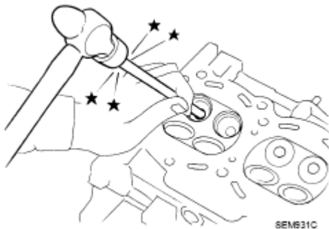
Fig. 202: Removing Valve Guide Using Hammer Courtesy of NISSAN MOTOR CO., U.S.A.
