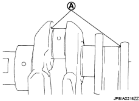
Fig. 265: Identifying Fillet Area Crankshaft Courtesy of NISSAN NORTH AMERICA, INC.
