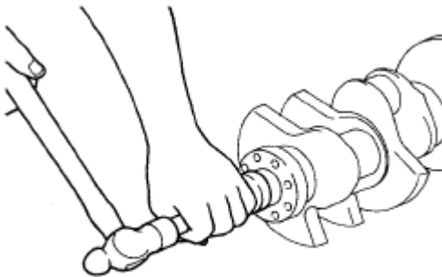
Fig. 209: Installing Crankshaft To Cylinder Block Using Suitable Tool
