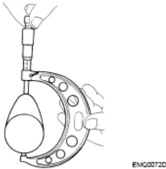
Fig. 156: Measuring Camshaft Cam Height Using Micrometer Courtesy of NISSAN NORTH AMERICA, INC.
