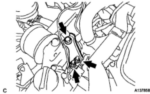
Fig. 37: Locating Engine Mounting Stay Bolt And Nut RH Courtesy of TOYOTA MOTOR SALES, U.S.A., INC.
