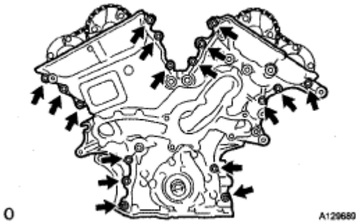
Fig. 164: Locating Timing Chain Cover Sub-Assembly Bolts And Nuts Courtesy of TOYOTA MOTOR SALES, U.S.A., INC.
