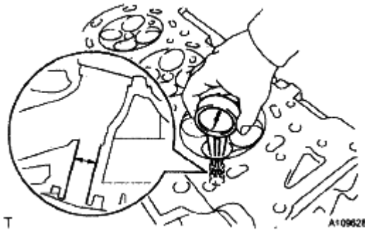
Fig. 317: Measuring Bush Bore Diameter Of Cylinder Head Courtesy of TOYOTA MOTOR SALES, U.S.A., INC.
