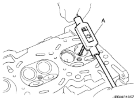
Fig. 183: Reaming Valve Guide Courtesy of NISSAN MOTOR CO., U.S.A.
