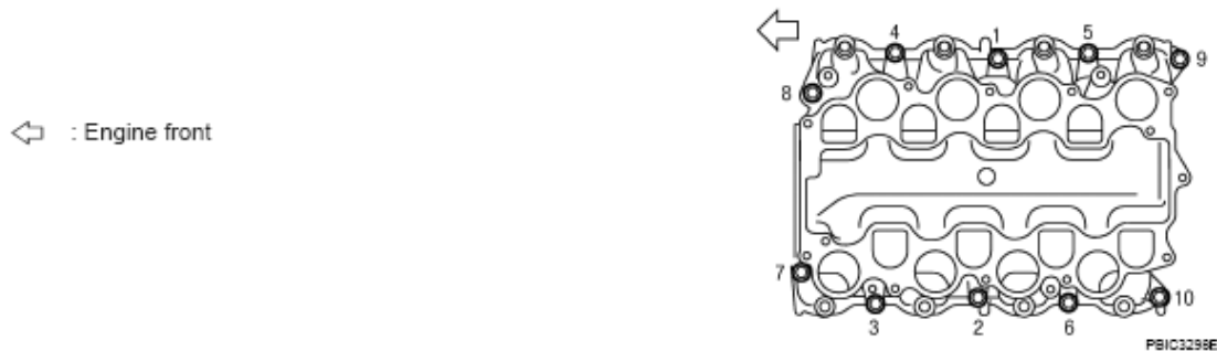
Fig. 19: Identifying Intake Manifold Bolt Loosening Sequence (Lower) Courtesy of NISSAN MOTOR CO., U.S.A.
