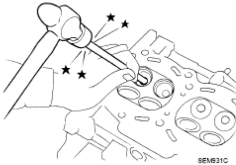
Fig. 157: Driving Out Valve Guide Courtesy of NISSAN MOTOR CO., U.S.A.
