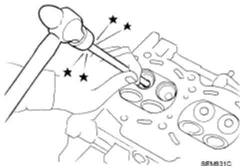
Fig. 161: Driving Out Valve Guide
