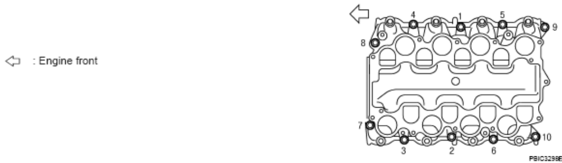
Fig. 16: Identifying Intake Manifold Bolts In Sequence (Lower) Courtesy of NISSAN MOTOR CO., U.S.A.
