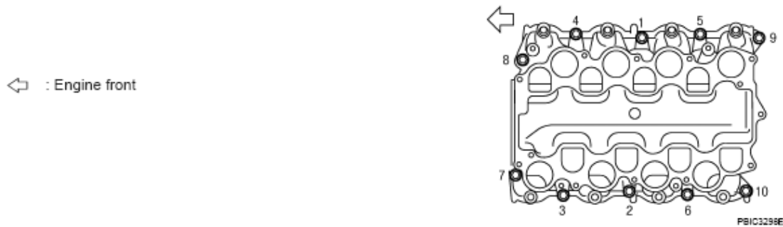
Fig. 18: Identifying Intake Manifold Bolts In Sequence (Lower) Courtesy of NISSAN MOTOR CO., U.S.A.
