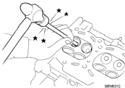
Fig. 147: Driving Out Valve Guide Courtesy of NISSAN MOTOR CO., U.S.A.
