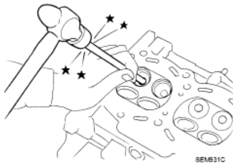
Fig. 154: Driving Out Valve Guide Courtesy of NISSAN MOTOR CO., U.S.A.
