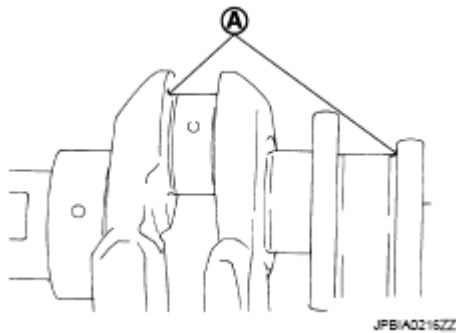
Fig. 313: Identifying Crankshaft Fillet Area Courtesy of NISSAN NORTH AMERICA, INC.
