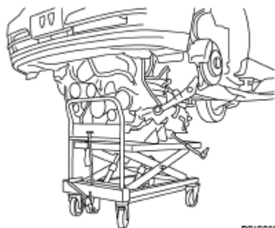
Fig. 140: Applying Manual Lift Table Caddy Courtesy of NISSAN NORTH AMERICA, INC.
