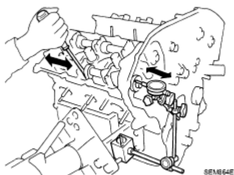
Fig. 204: Measuring Camshaft End Play Using Dial Indicator Courtesy of NISSAN NORTH AMERICA, INC.
