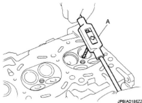
Fig. 225: Reaming Cylinder Head Valve Guide (EXH) Hole Using Valve Guide Reamer Courtesy of NISSAN NORTH AMERICA, INC.
