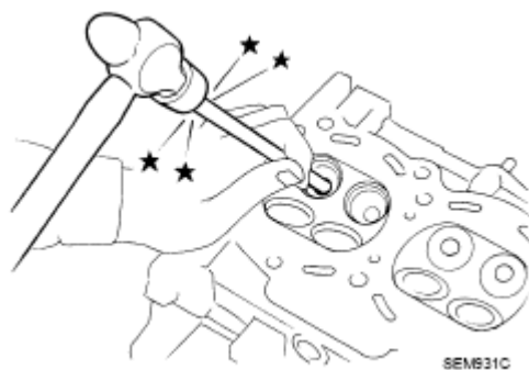
Fig. 224: Driving Out Valve Guide Using Press Courtesy of NISSAN NORTH AMERICA, INC.
