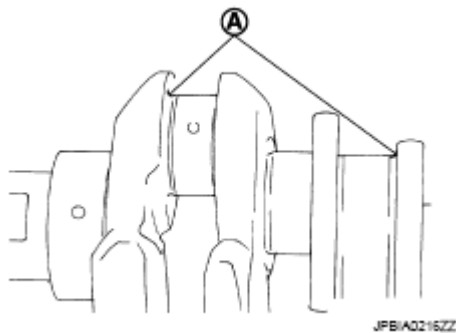
Fig. 306: Identifying Fillet Radius
