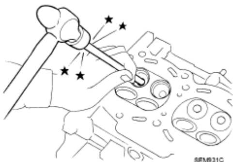
Fig. 216: Driving Out Valve Guide Using Tool
