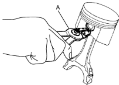
Fig. 240: Removing Snap Rings Using Snap Ring Plier Courtesy of NISSAN NORTH AMERICA, INC.
