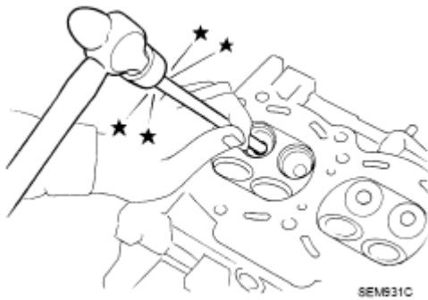
Fig. 216: Removing Valve Guide Using Hammer And Valve Guide Drift Courtesy of NISSAN MOTOR CO., U.S.A.
