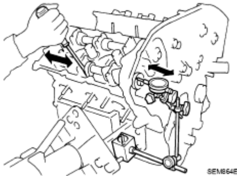
Fig. 196: Measuring Camshaft End Play Courtesy of NISSAN MOTOR CO., U.S.A.
