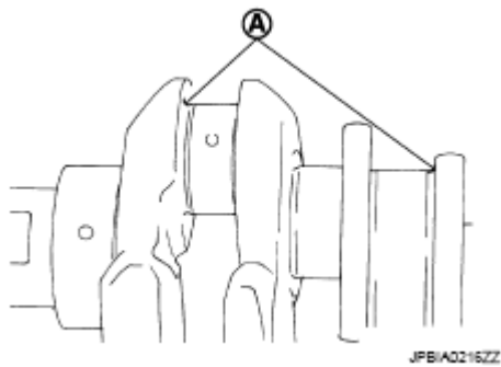
Fig. 306: Identifying Crankshaft Fillet R Courtesy of NISSAN MOTOR CO., U.S.A.
