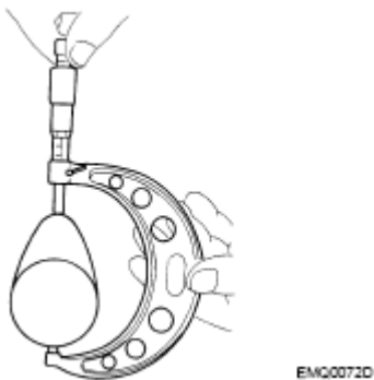
Fig. 193: Checking Camshaft (EX) Cam Height Courtesy of NISSAN MOTOR CO., U.S.A.
