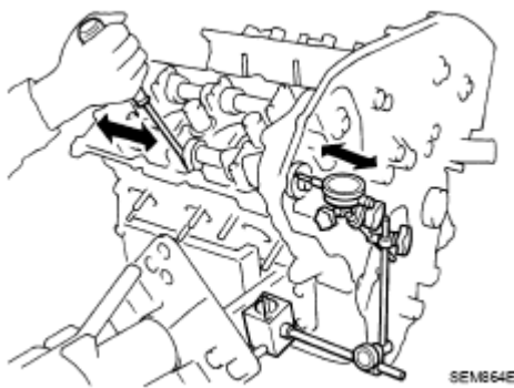
Fig. 196: Checking Camshaft (EX) End Play Courtesy of NISSAN MOTOR CO., U.S.A.
