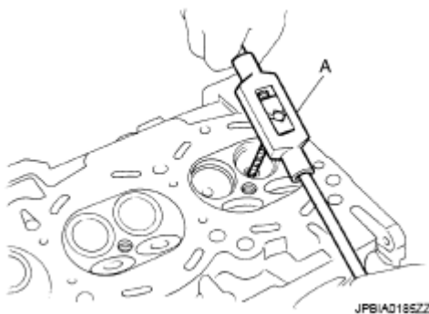
Fig. 217: Reaming Cylinder Head Valve Guide (EX) Hole Courtesy of NISSAN MOTOR CO., U.S.A.
