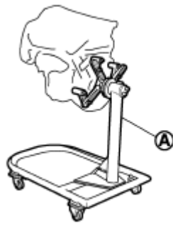
Fig. 139: Holding Mating Surface Of Transmission With Drive Plate (A/T Models) Or Flywheel (M/T Models) Using Engine Stand Courtesy of NISSAN MOTOR CO., U.S.A.
