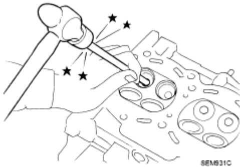
Fig. 216: View Of Driving Out Valve Guide Courtesy of NISSAN MOTOR CO., U.S.A.
