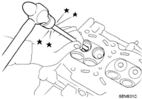
Fig. 192: Driving Out Valve Guide Using Press Courtesy of NISSAN NORTH AMERICA, INC.
