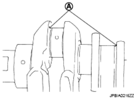
Fig. 289: Identifying Connecting Rod Bearing Courtesy of NISSAN MOTOR CO., U.S.A.
