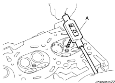
Fig. 230: Reaming Cylinder Head Valve Guide (EXH) Hole Courtesy of NISSAN MOTOR CO., U.S.A.
