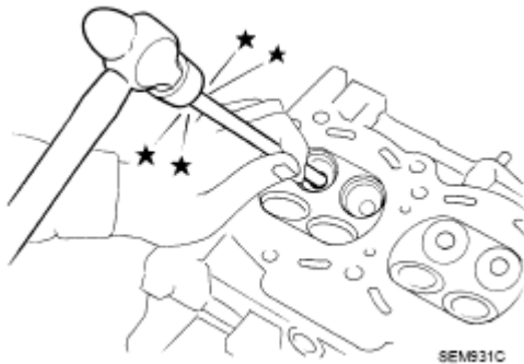
Fig. 229: Driving Out Valve Guide Courtesy of NISSAN MOTOR CO., U.S.A.
