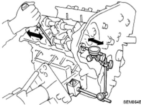
Fig. 181: Measuring Camshaft End Play Courtesy of NISSAN MOTOR CO., U.S.A.
