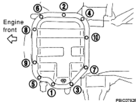
Fig. 48: Identifying Oil Pan (Lower) Bolts Tightening Sequence Courtesy of NISSAN MOTOR CO., U.S.A.
