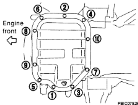
Fig. 50: Identifying Oil Pan (Lower) Bolts Loosening Sequence Courtesy of NISSAN MOTOR CO., U.S.A.
