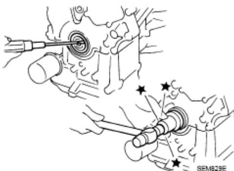
Fig. 213: Identifying Front Oil Seal Courtesy of NISSAN MOTOR CO., U.S.A.
