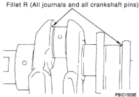
Fig. 299: Identifying Crankshaft Journals And Crankshaft Pins Courtesy of NISSAN MOTOR CO., U.S.A.
