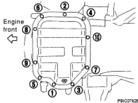
Fig. 66: Identifying Oil Pan (Lower) Bolts Tightening Sequence Courtesy of NISSAN MOTOR CO., U.S.A.
