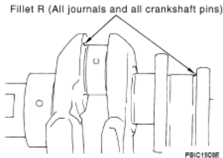
Fig. 295: Identifying Crankshaft Journals And Crankshaft Pins Courtesy of NISSAN MOTOR CO., U.S.A.
