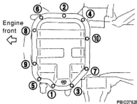
Fig. 35: Identifying Oil Pan (Lower) Bolts Loosening Sequence Courtesy of NISSAN MOTOR CO., U.S.A.
