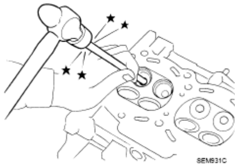
Fig. 235: Driving Out Valve Guide
