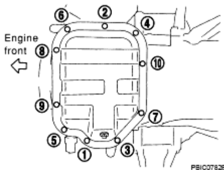
Fig. 49: Identifying Oil Pan (Lower) Bolts Loosening Sequence
