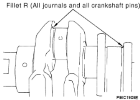
Fig. 294: Identifying Crankshaft Journals And Crankshaft Pins
