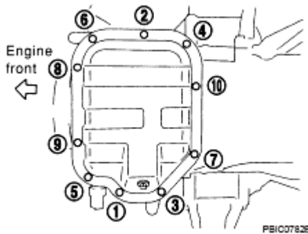
Fig. 34: Identifying Oil Pan (Lower) Bolts Loosening Sequence
