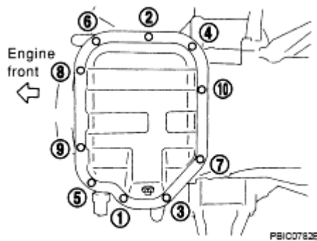
Fig. 47: Identifying Oil Pan (Lower) Bolts Tightening Sequence
