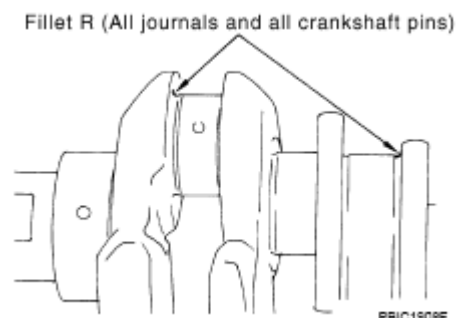
Fig. 298: Identifying Crankshaft Journals And Crankshaft Pins
