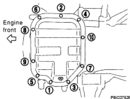
Fig. 65: Identifying Oil Pan (Lower) Bolts Tightening Sequence
