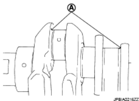
Fig. 291: Identifying Crankshaft Pin Courtesy of NISSAN MOTOR CO., U.S.A.
