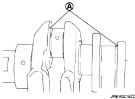
Fig. 295: Identifying Crankshaft Pin Courtesy of NISSAN MOTOR CO., U.S.A.
