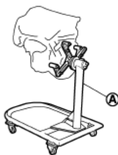
Fig. 165: Holding Mating Surface Of Transmission With Drive Plate Courtesy of NISSAN MOTOR CO., U.S.A.
