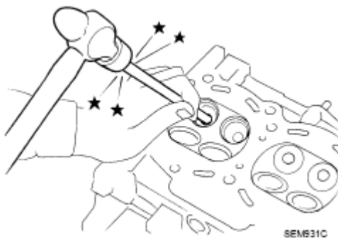
Fig. 204: Driving Out Valve Guide
