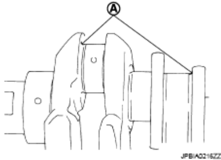
Fig. 292: Identifying Crankshaft Pin
