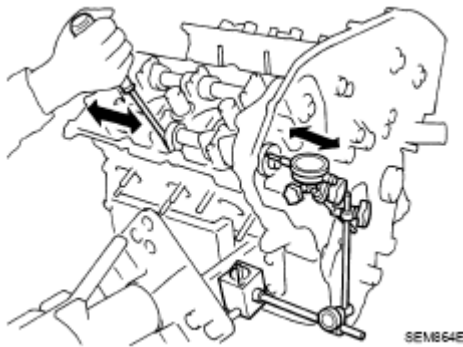
Fig. 133: Measuring Camshaft End Play
