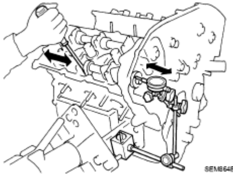
Fig. 141: Checking Camshaft End Play Courtesy of NISSAN MOTOR CO., U.S.A.
