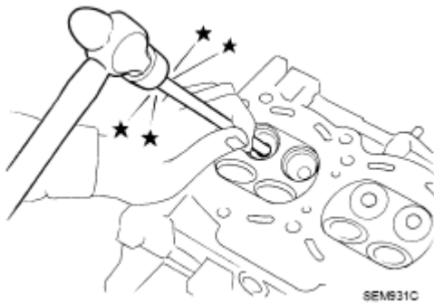
Fig. 207: Pressing Valve Guide Courtesy of NISSAN MOTOR CO., U.S.A.
