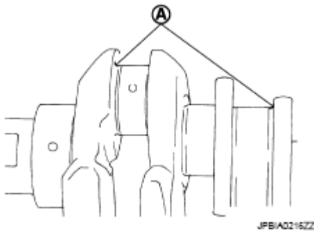
Fig. 296: Identifying Crankshaft Main Journal Courtesy of NISSAN MOTOR CO., U.S.A.
