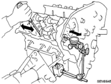
Fig. 180: Measuring End Play Of Dial Indicator Courtesy of NISSAN MOTOR CO., U.S.A.
