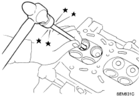
Fig. 235: Driving Out Valve Guide
