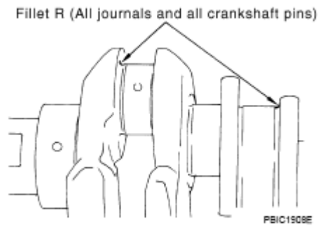
Fig. 305: Identifying Crankshaft Journals Courtesy of NISSAN MOTOR CO., U.S.A.
