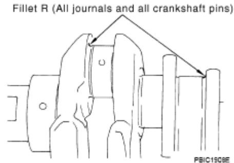
Fig. 301: Identifying Crankshaft Journals Courtesy of NISSAN MOTOR CO., U.S.A.
