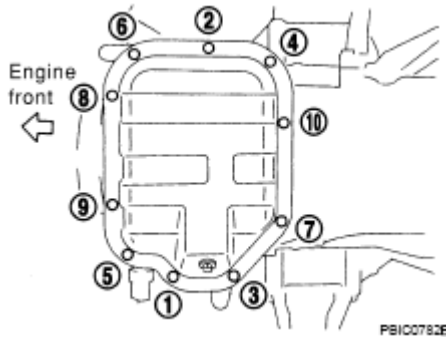
Fig. 34: Loosening And Tightening Oil Pan Mounting Bolts In Sequence (Lower) Courtesy of NISSAN MOTOR CO., U.S.A.
