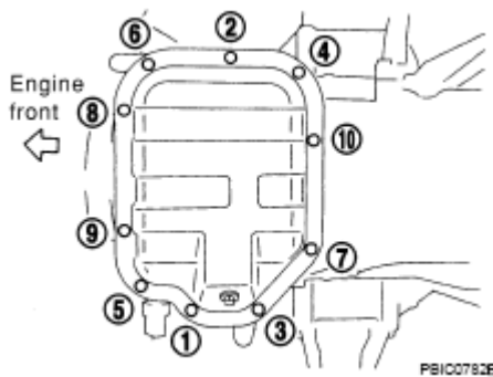
Fig. 47: Loosening And Tightening Oil Pan Mounting Bolts In Sequence (Lower) Courtesy of NISSAN MOTOR CO., U.S.A.
