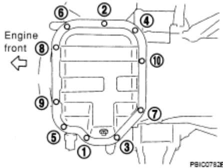
Fig. 65: Loosening And Tightening Oil Pan Mounting Bolts In Sequence (Lower) Courtesy of NISSAN MOTOR CO., U.S.A.
