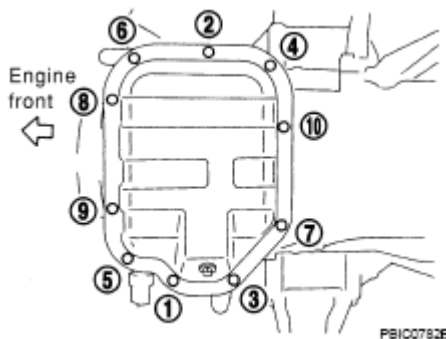
Fig. 49: Loosening And Tightening Oil Pan Mounting Bolts In Sequence (Lower) Courtesy of NISSAN MOTOR CO., U.S.A.
