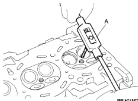
Fig. 209: Reaming Cylinder Head Valve Guide Hole Courtesy of NISSAN MOTOR CO., U.S.A.
