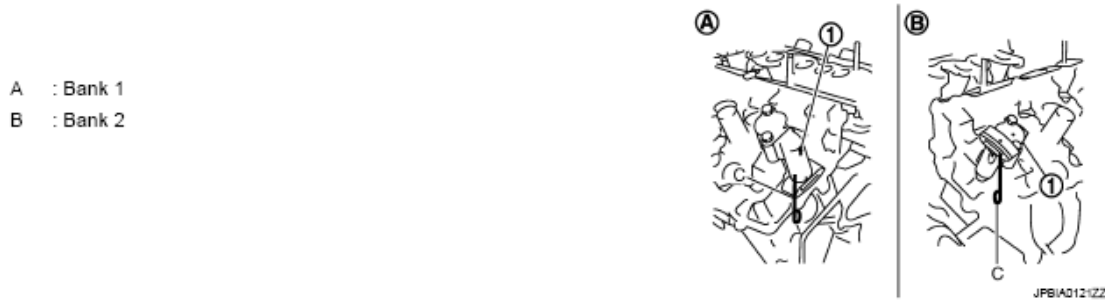
Fig. 124: Identifying Timing Chain Tensioners With Stopper Pin Courtesy of NISSAN MOTOR CO., U.S.A.
