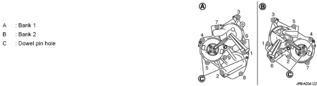
Fig. 118: Identifying Mounting Bolts Tightening Sequence Courtesy of NISSAN MOTOR CO., U.S.A.
