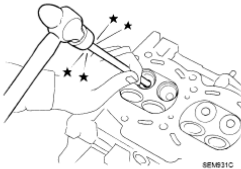
Fig. 204: Tapping Valve Guide With Press & Hammer Courtesy of NISSAN MOTOR CO., U.S.A.
