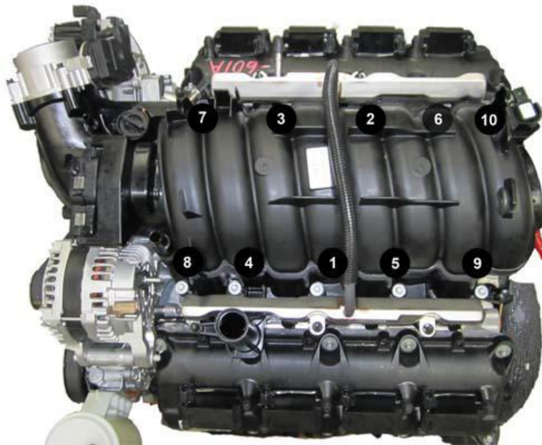
Fig. 72: Intake Manifold Removal/Installation Sequence
