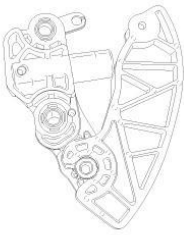
Fig. 410: Timing Chain Tensioner Arm Courtesy of CHRYSLER GROUP, LLC
