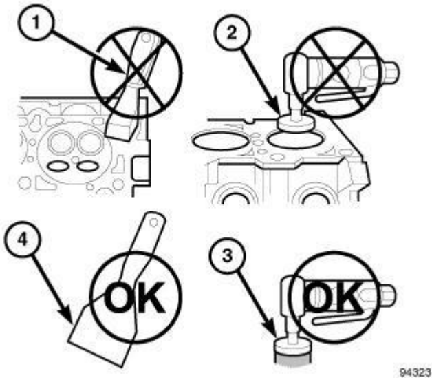
Fig. 4: Proper Tool Usage For Surface Preparation Courtesy of CHRYSLER GROUP, LLC
