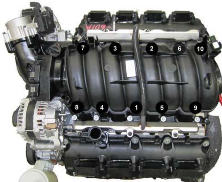
Fig. 29: Intake Manifold Removal/Installation Sequence Courtesy of CHRYSLER GROUP, LLC
