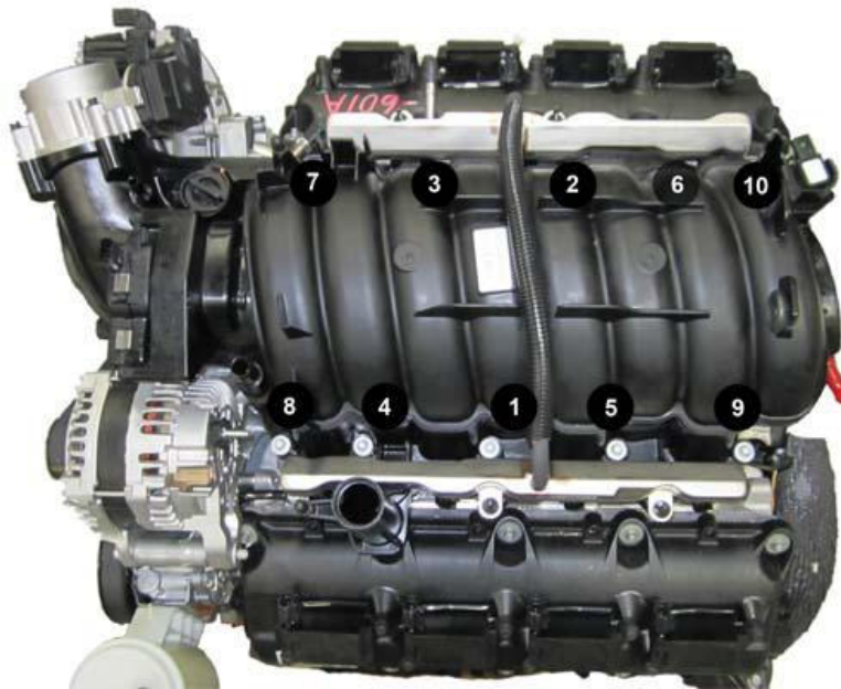
Fig. 343: Intake Manifold Removal/Installation Sequence Courtesy of CHRYSLER GROUP, LLC
