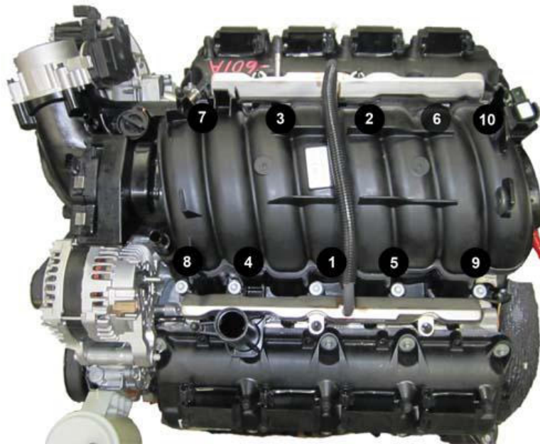
Fig. 47: Intake Manifold Removal/Installation Sequence Courtesy of CHRYSLER GROUP, LLC
