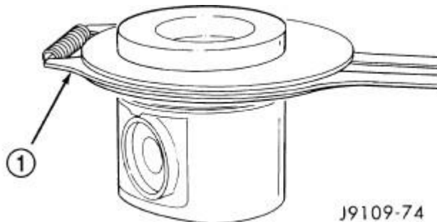
Fig. 154: Piston Ring Installation Tool Courtesy of CHRYSLER GROUP, LLC
