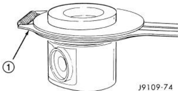
Fig. 154: Piston Ring Installation Tool Courtesy of CHRYSLER GROUP, LLC
