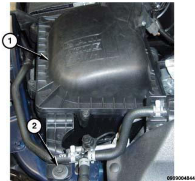
Fig. 29: Intake Air Housing & Bolt
