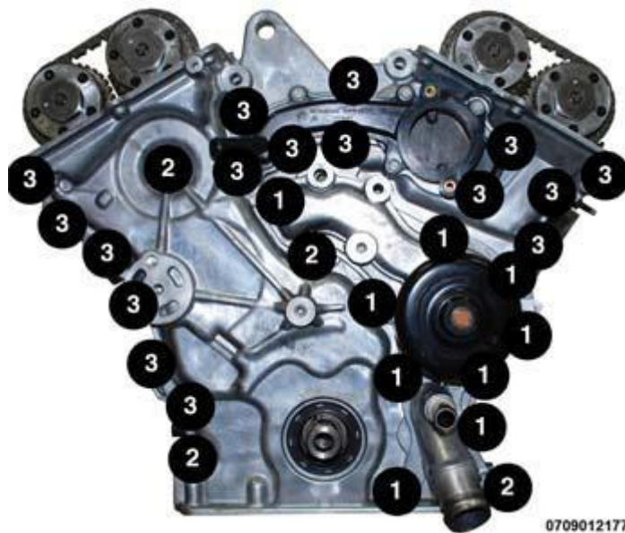
Fig. 654: Engine Timing Cover(s) Bolts Tightening Sequence Courtesy of CHRYSLER GROUP, LLC
